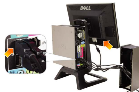
7 Connect the USB, keyboard and mouse cables to the computer as shown
